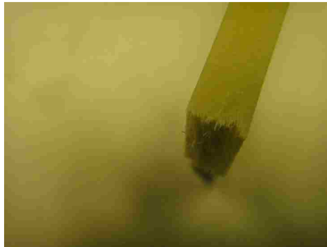
Figure 72: Post failure analysis of fiber orientation
