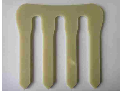
Figure 65: Final shear tie
