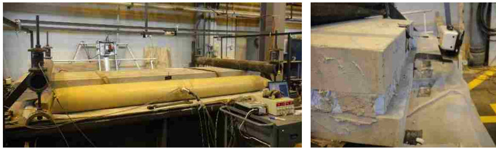
Figure 37: Center-span displacement and end-slip instrumentation
