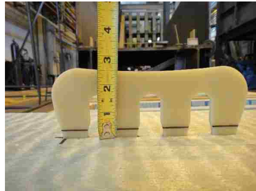
Figure 66: Fabrication of test specimen
