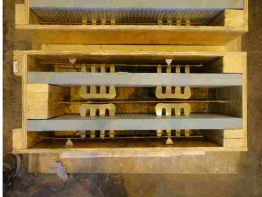
Shear tie placed through XPS
