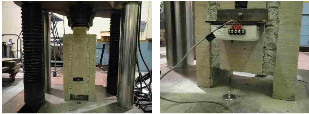
Figure 68: New double shear test setup and string potentiometer
